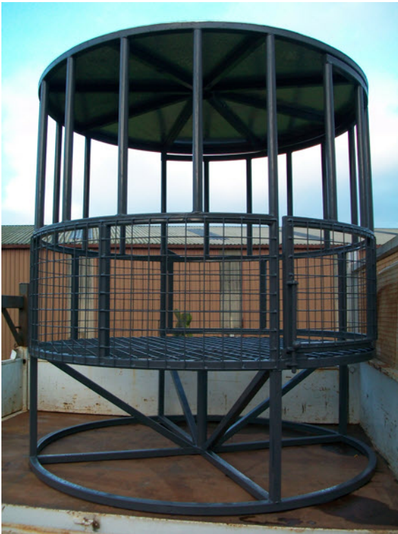
Photograph 3. The feeder for horses. The upper section is in two parts, one of which is hinged. The bale, which weighs about 600Kg is loaded from the side by tractor or teleporter.
