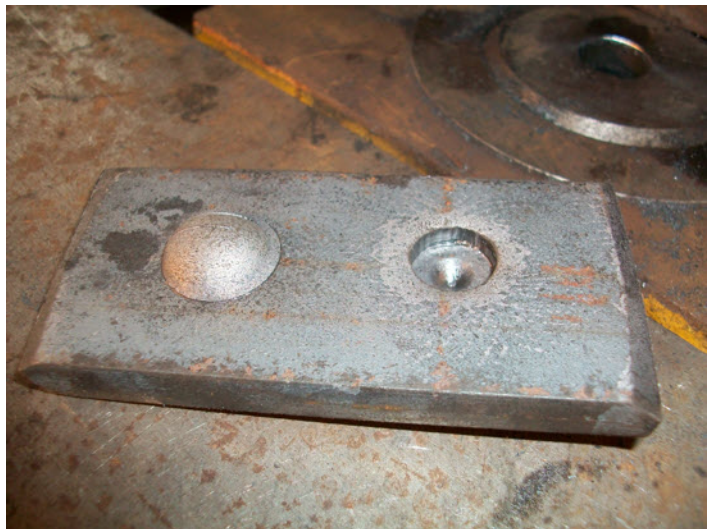
Photograph 4. A sample of the simulated rivet. The punch has penetrated to about half of the thickness of the metal. The die has a larger diameter than the punch. Since the underside of the workpiece is not supported as it would normally be, the steel is stretched into a dome as shown in the example formed from the opposite side of the test piece.
