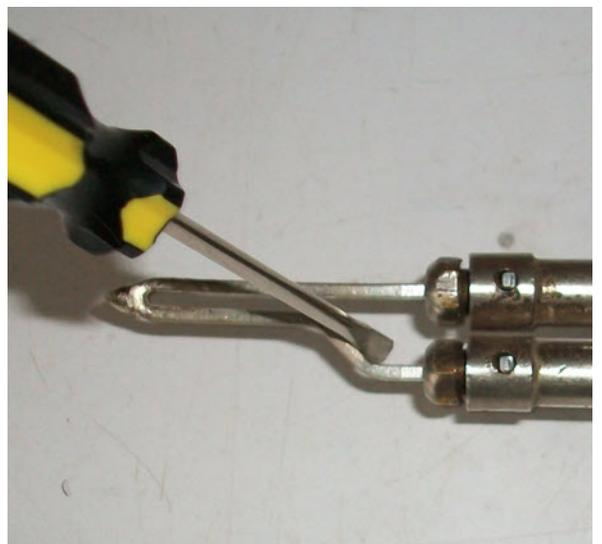
Photo 2. The screwdriver will vibrate in sympathy with the alternating magnetic field when the blade is held in close proximity to the soldering tip.
