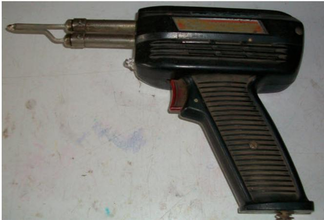
Photo 1. My “Weller” soldering gun after 45 years of regular use. The tip reaches operating temperature within a few seconds.
