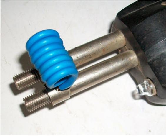
Photo 3. The degaussing effect is enhanced by making a multi-turn coil. If desired, more than one layer of turns can be employed.
