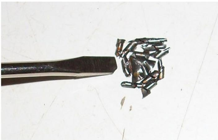
Photo 5. What this photograph cannot show is that there is no tendency for the swarf to stick together or be attracted to the screwdriver, once both have been degaussified.
