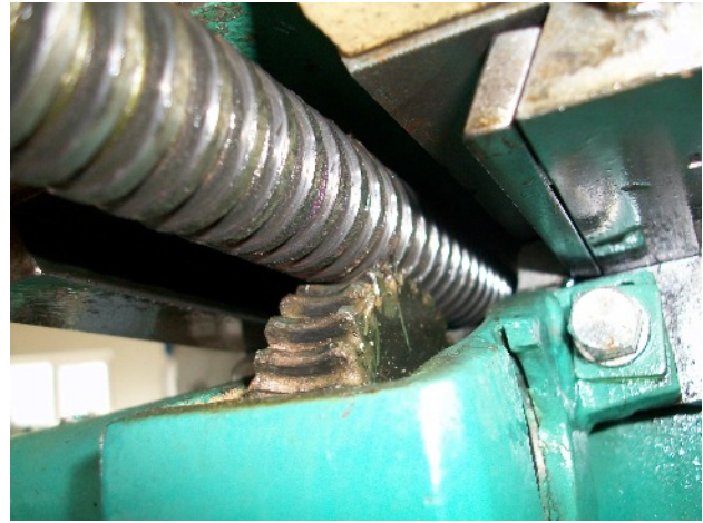
Photo 2. A view from beneath the table showing the worm and wormwheel arrangement.
