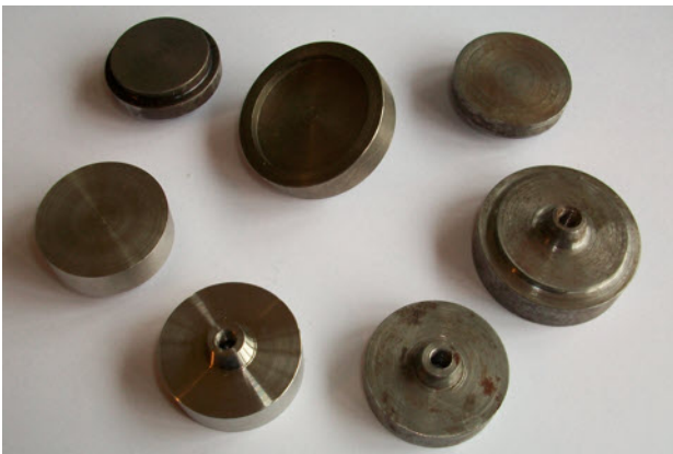
Photograph 1. Some of the stainless steel sample holders intended for the rheometer. Several have been used and remain contaminated with polymer residue.
