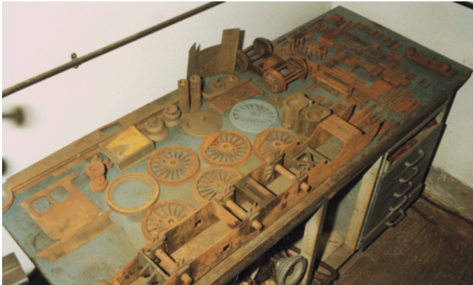
Photo 6. The components of the 5" gauge Springbok locomotive set out prior to sale. Many smaller parts had corroded beyond recovery and were discarded. The die holder pictured to the right of the cab side is the one item I retained.
