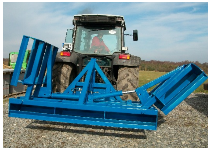
Photo 1. Bill unfolds a land leveller which Mike had just designed and built for a customer who was too mean to have the job galvanised.
