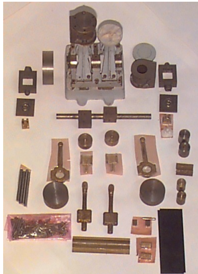
Photo 5. The Stuart D10 as it was sold. The bedplate, columns and cylinders had been machined along with the top cylinder covers. The valve chests and cover plates were partly machined. No work had been carried out on any of the moving parts.
