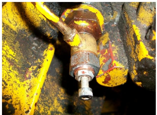
*Photo 8: The banjo reinstalled in the relief valve of the Petter. Oil flow to the rockers was easily controlled by adjusting the setscrew.*
