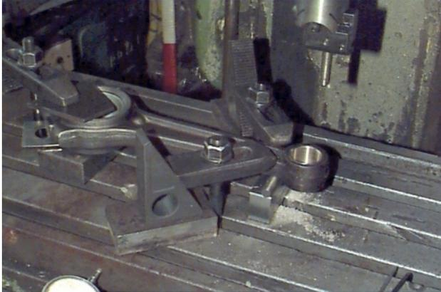
*Photo 5: One of the Petter conrods has its small end bored to size on the Cincinnati Mill*
