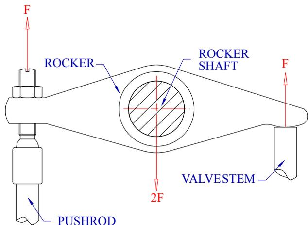
*Drawing 1: The popular design of pushrod type valve gear is such that the bearing load is carried by the lower half of the rocker shaft.*
