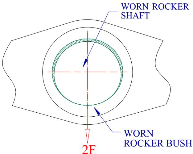
*Drawing 3: The approximately ellipsoidal form of a worn shaft and bush represents a more favourable load distribution than is obtained from small cylindrical components.*
