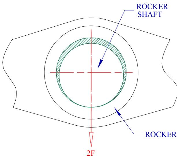
*Drawing 2: Clearance between the shaft and rocker permits the lubricant to be displaced from the area where it is most needed. An oscillating component does not benefit from induced hydrodynamic lift to the same extent as one which rotates continuously.*
