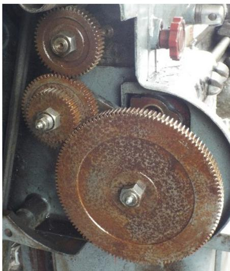
Photo 2. The incorrect gear train.
