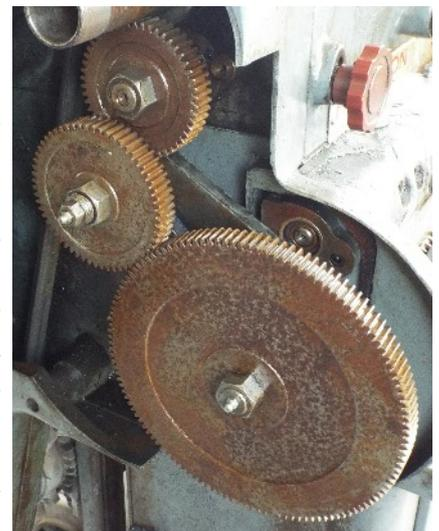
Photo 3. The “Correct” gear train.
