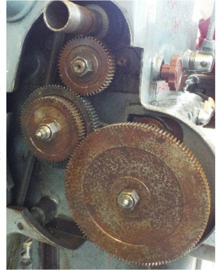
Photo 4. A sensible gear train for metric pitches on my L5.
