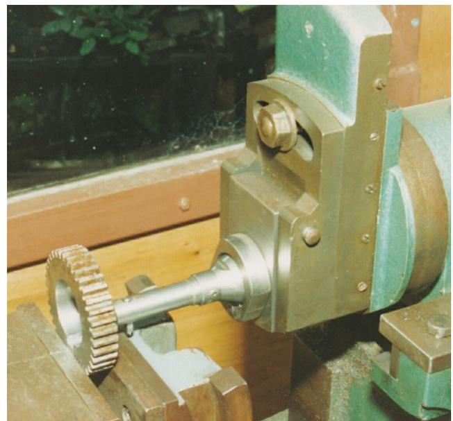
Photo 3. Cutting a keyway in a gear.
