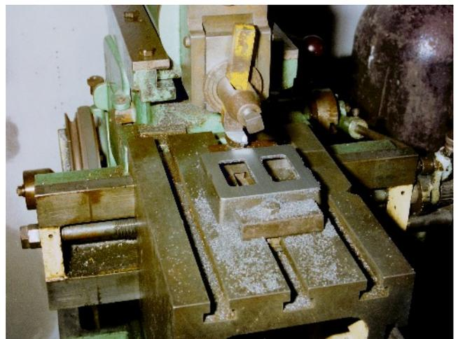
*Photo 2. Shaping the top of a Stuart Double 10 stationary steam engine bedplate.*
