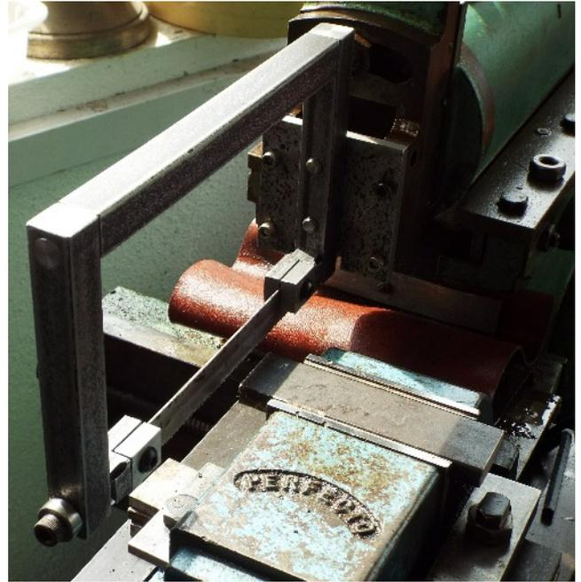
*Photo 5. The shaper takes the strain out of hacksawing and brings a high degree of accuracy to the process.*
