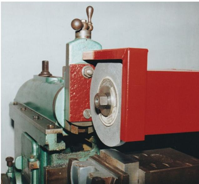
*Photo 4. The shaper rigged as a surface grinder.*
