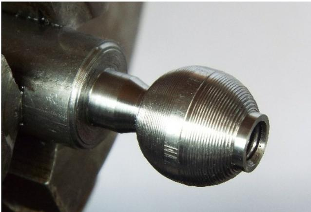
*Photo 1. A ball handle produced by coordinate machining prior to finishing with a file and abrasive paper.*
