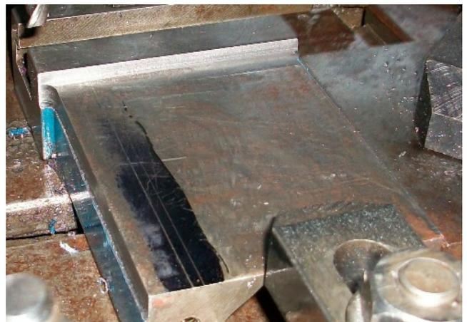
*Photo 4. The slide was mounted with the scribed line parallel to the milling table cross feed. Datum faces were machined along the left hand edge of the slide and to the rear of the T slot.*
