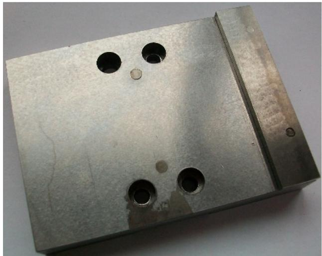
*Photo 6. The mounting plate prior to drilling the holes for securing to the compound slide. Dowels for the toolholder block and the datum strip are visible.*
