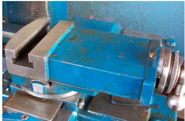
*Photo 2. The Little John topslide is not particularly attractive, but what it lacks in beauty is more than offset by its sturdiness and ease of modification. Good engineering doesn't have to "Look right" to be right.*
