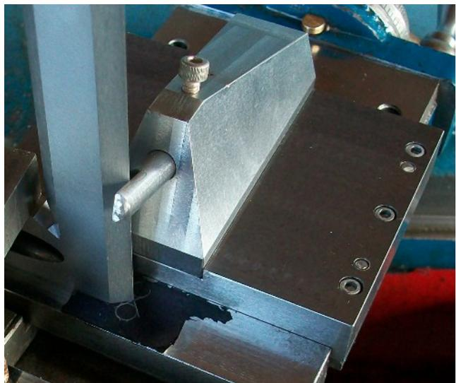
*Photo 7. The try square was aligned with the axis of rotation of the compound slide. Clearance between the gauge rod held in the toolholder and the edge of the try square was measured. The datum strip secured along the side of the baseplate had a machining allowance from which the appropriate amount was removed by grinding.*
