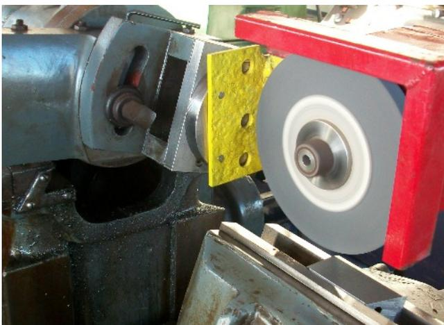
*Photo 5. The head on the shaper is rotated to within about 5 degrees of horizontal, providing sensitive height adjustment during grinding operations.*
