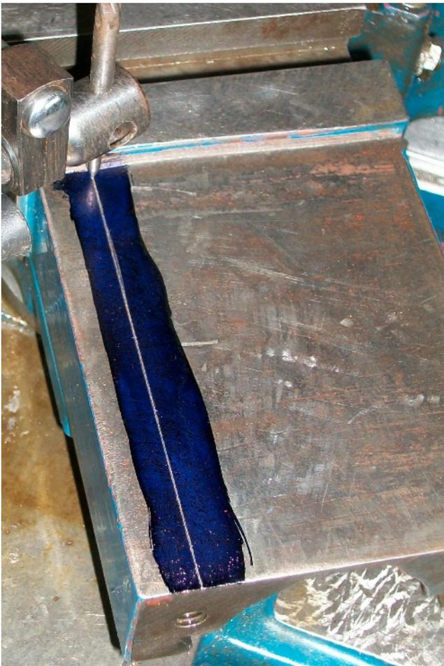
*Photo 3. With the paint removed it was evident that the topslide had been rough machined. Machine marks were cleaned by scraping. Note the reduced thickness of the slide in the central region visible at the end. The scribed line is parallel to the line of travel of the slide.*
