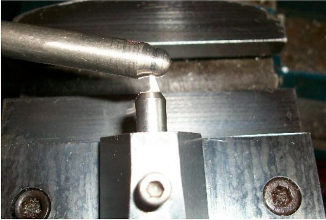
*Photo 8. The spherical turning tool having machined a ball end on a test piece. Note the excessive overhang of the work.*
